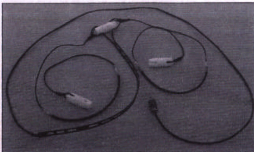
Photo A— Full view of the W5GI Multiband Mystery Antenna, with all sections shorted considerably for illustration.
