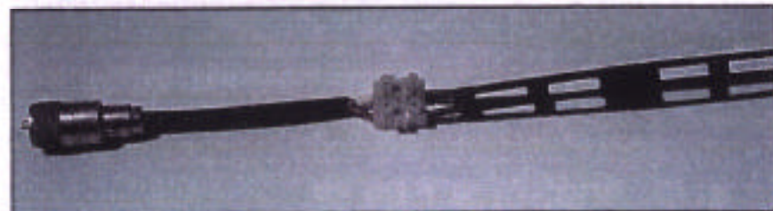
Photo E— Connection of twinlead to coax. Short length of coax section is for illustration only. All connections should be weatherproofed with shrink-tubing, CoaxSeal®, or similar.
