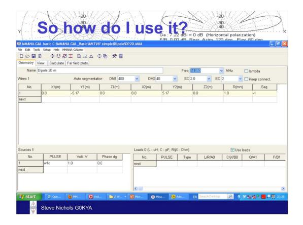
Here I have made a dipole. It is 10.34m (2 x 5.17m) long with wire of radius 1mm. We are feeding it in the middle (w1c – wire 1, centre). There are no loading coils or traps. Just leave the auto segmentation as it is
