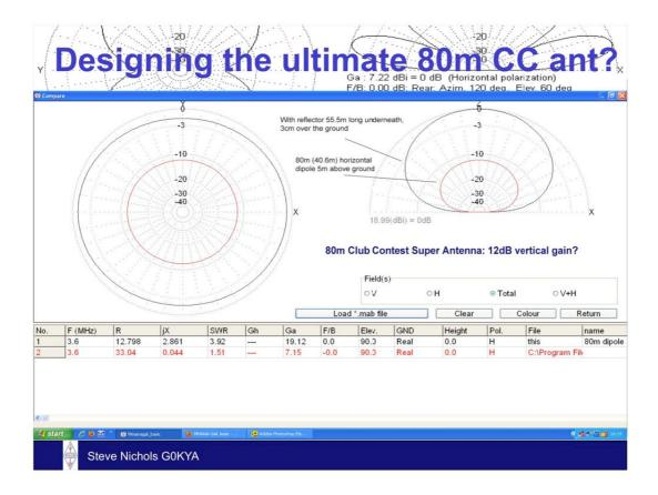
Putting a 55.5m reflector just 3cm off the ground under an 80m horizontal dipole could give great NVIS gain if the model is to be believed. But does it? It is still to be tried.
