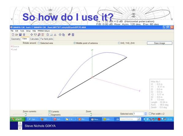
This is the current distribution on the dipole. The little red blob in the middle is the feedpoint. We can see the current maximum (which does the radiating) is in the centre.
