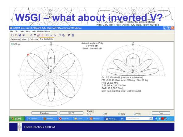
Note the nice petal-shaped predicted radiation pattern for a flattop-mounted W5GI Mystery Antenna
