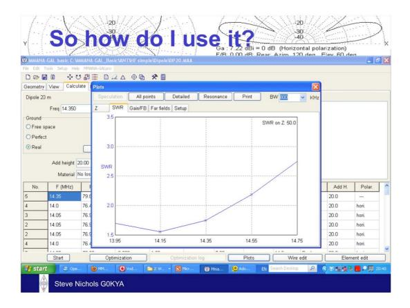
You can get a simulated SWR curve – your measured result may be better at the end of a length of coax due to losses. Note impedance is 50 Ohms.
