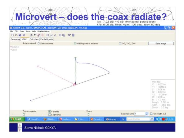
You can see the prediction is that the coax does most of the radiation – that's where the maximum current is. To be fair, the antenna is designed to include the feeder as part of the overall antenna system..
