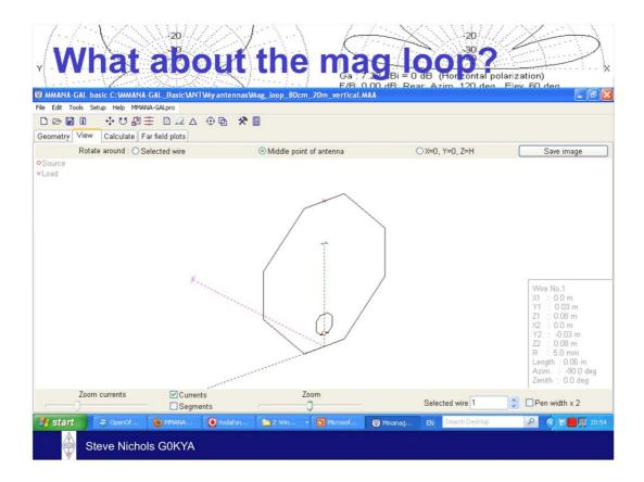
You can model mag loops using straight sections – this model comes with the package.
