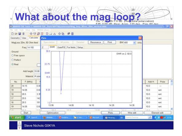
Note the sharp SWR and narrow bandwidth of a mag loop at its resonant frequency.
