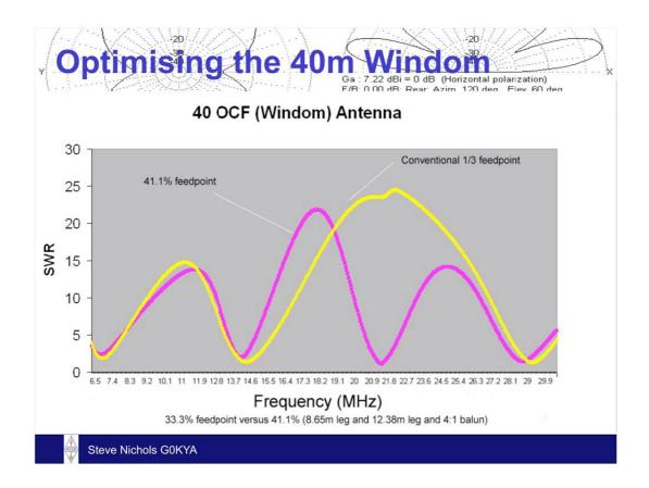
Here you can see that feeding a 40m Windom at a special point (not the one third/two third point) gives you 15m too. These results were output from MMANA-GAL and then imported into a spreadsheet. The 8.65m/12.38m OCF Windom gives you 40m, 20m, 15m and 10m. That is, you gain 15m.
