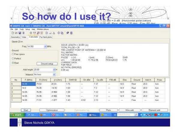
Here we placed it 20m above ground and ran it at a number of frequencies in the 20m band. You can see the modelled SWR varies 1.43:1 to 1.75:1 Maximum gain is at 14.6 degrees to the horizon. Note: I forget to specify copper wire – it is assuming no losses in the wire.
