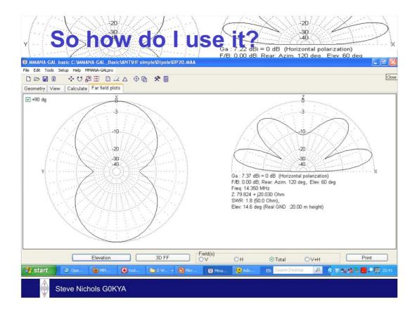
These are the predicted radiation patterns – left hand is looking down on the antenna. Make sure you set the elevation angle you wish to view – this is at the 14.6 degrees maximum. You can select vertical or horizontal polarisation or total radiation.
