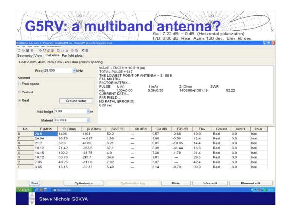
As an example, this is a run on a simulated G5RV antenna. As you can see the predicted SWR figures are not very low on most bands. So is it a true multiband antenna?
