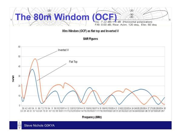
This is a model of the classic 80m Windom (off centre fed dipole) antenna – 136ft (11.82m one leg, 29.63m the other – fed with a 4:1 balun). You can see the low SWR points when mounted flat top.
