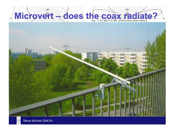
The Microvert is a tiny antenna fed with a quarter wave of coax to which you only connect the inner. You have a choke at the other end of the coax.
