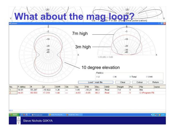
You can see how the radiation pattern may change as a vertical mag loop is raised. It might be better all round at 3m and not 7m according to the model.
