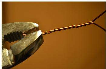
measuring out two pieces of 20SWG enamelled copper wire – one is about 1m, long and the other about 22cm. Twist the two together for the first 130mm, ensuring that you do this neatly. The twisted section then makes up the two bifilar turns on the primary.
