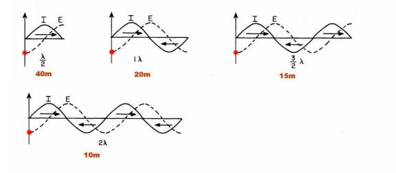
How the antenna works as a multiple of half wave lengths on the higher bands:
