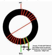
somewhere between 2000-5000 Ohms. In some designs, my earlier ones included, we make a resonant circuit using a toroid coil and capacitor to resonate at the frequency required.
