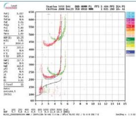
This Chilton Digisonde image clearly shows the critical frequency of the extraordinary wave (green) is higher than the ordinary wave (red) by about 0.7MHz. 5MHz was probably open to stations around the UK at this time.
