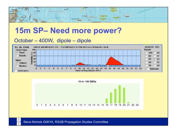
The problem with the higher bands is that the solar cycle has not really been playing ball – the solar flux has not really been high enough very often to provide good, reliable DX openings. It may therefore be a bit of a lottery.
