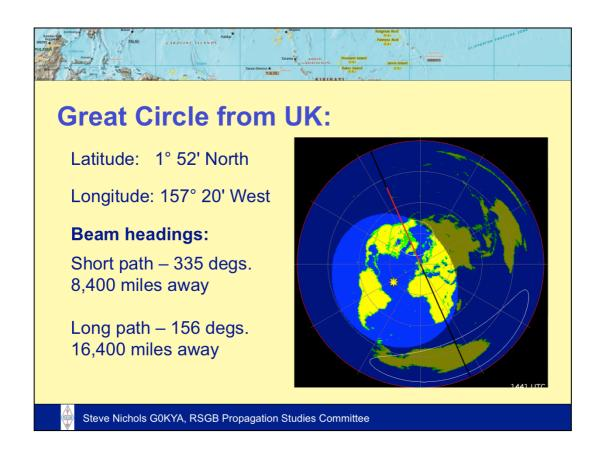
This highlights the first propagation problem – Kiritimati lies on a beam heading of about 335 degrees from the UK which puts our signals slap bang through the auroral oval around the north pole. Conversely, the long path heading of 156 degrees (and 16,400 miles) goes through the south auroral oval.
