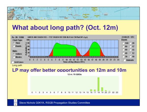
You may get much stronger signals on 12m and 10m via the long path. T32C will start to concentrate more on long path to the UK and will be installing a new high dipole.
