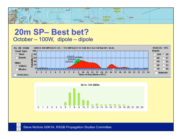
This band will be chocaful of stations trying to work T32C and perversely may prove to be one of the hardest bands to work them. The band will be open for a longer period than the lower bands, but will peak at around 0730 -1200UTC. Signals (if there at all) will then take a bit of dive before the possibility of another short opening around 1600-1700UTC.
