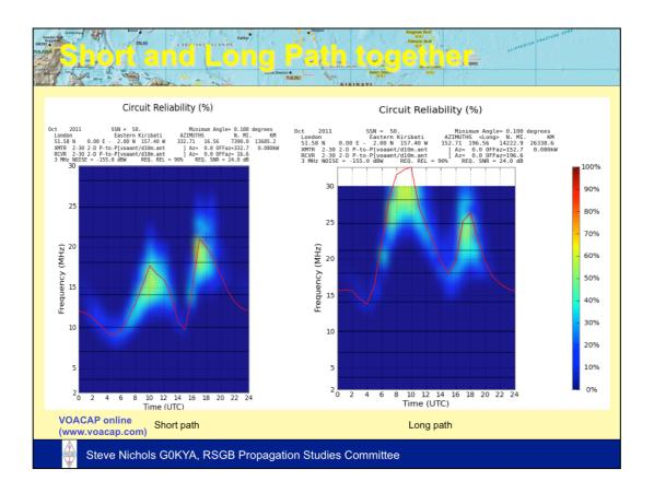
Short path on left, long path on right. Produced using VOACAP online. Note the higher MUFs on long path, but overall greater probability of openings on short path.
